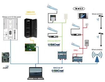
Cristal Controls offers completely integrated lighting control solutions with its proprietary Jasper multi-purpose energy management software and the latest in DALI dimming control and individual fixture addressability technology.
